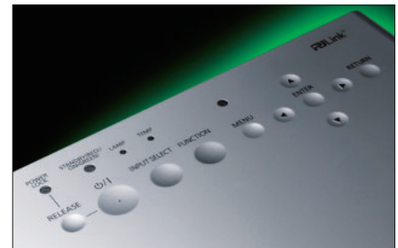
Touch-sensor controls on the top.
